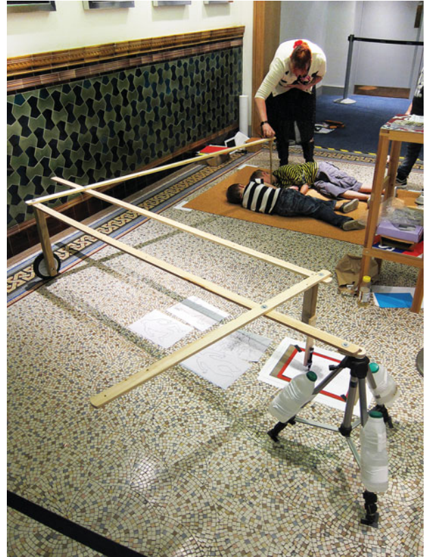
Figure 9. Nick Sayers, Giant Pantograph , 2011. Photograph of 2-m pantograph body drawing machine, Wood, nuts and bolts, photographic tripod, art paper, mechanical pencil.
